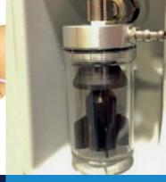
Place the collection reservoir into the reservoir holder. Attach a vacuum line to the yellow-capped port on the collection reservoir.
